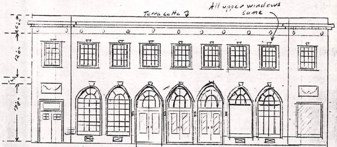
Pressed face brick all exterior walls Terra cotta trim and coping Front Elevation
