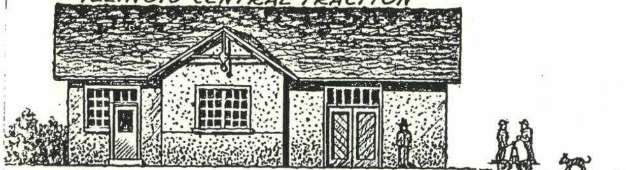
TRACK-SIDE FAÇADE OF WABASH DEPOT AT HARRIS TOWN, ILL. STUCCOED OVER WOOD, ALL GREY PAINTED. REFER TO PL. NO. 32.
