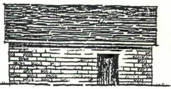
•TRACK-SIDE ELEVATION. - Fogarty Sub-Station - 2,000 AMPERES-AUTOMATIC. CONSTRUCTED AFTER 1934. SIMPLE CONCRETE BLOCK STRUCTURE - C. 12' X 20'
